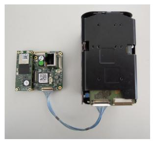
Connect the other connectors according to your needs (Ethernet, HDMI, GPIO, debug cable, Wi-Fi Antenna
