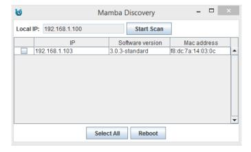
It works sending a JSON message to a specific multicast address, Mamba will respond with its own IP address, software version and MAC address.
