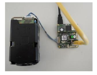
Connect the power supply to the 2-pins connector. The maximum voltage is 12V.
